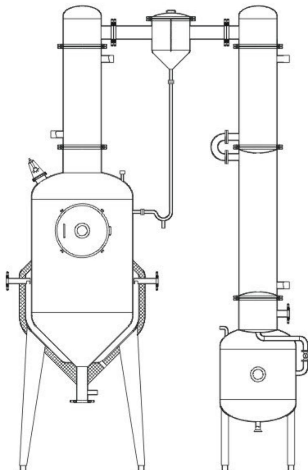
The device includes concentration tank、condensator、gas-liquid separator、cooler and liquid receiving barrel. The concentrator tank is of clip sleeve structure. The condensator is of line pipe type and the cooler is of tray pipe type. The device is suitable to concentrate in the pharmacy、foodstuff and chemistry and simple reflux extraction. The fact that the part in contact with the material is made with stainless steel brings qualified anti-corrosion performance, meeting with the GMP standard.
